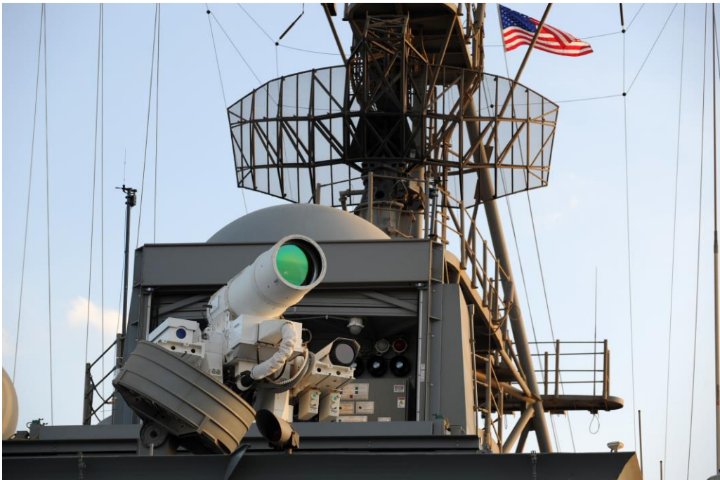
Fig. 2. AN/SEQ-3 Laser Weapon System (LaWS) aboard USS Ponce
